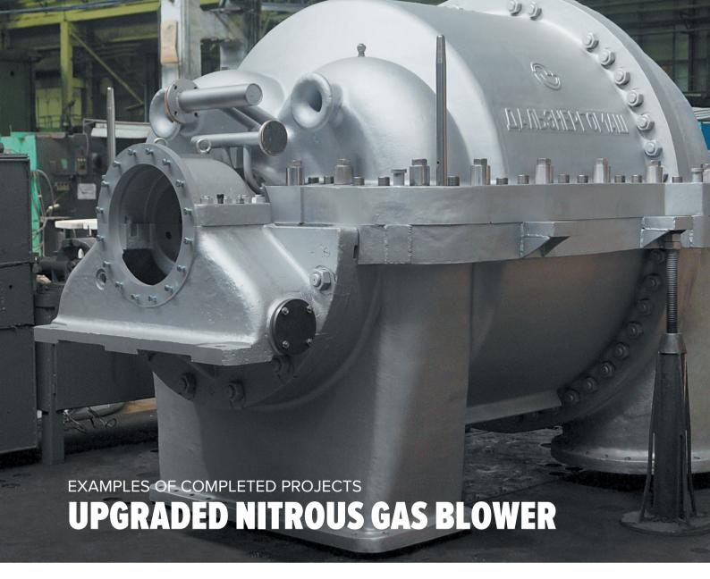
The final assembly stage of a nitrous gas upgraded blower 1150-42-1 at the plant 'Dalenergomash'
