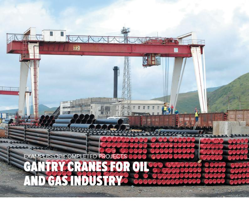
By order of Joint Venture 'Sakhalin – Shelf – Service' LLC six heavy-duty gantry cranes with lifting capacity of 20 and 32 tons, span 32 m, height 14 m have been manufactured and mounted for unloading, stocking, and rehandling of large diameter pipes for construction of oil and gas pipe lines on a cargo area of Kholmsk fishing port.
