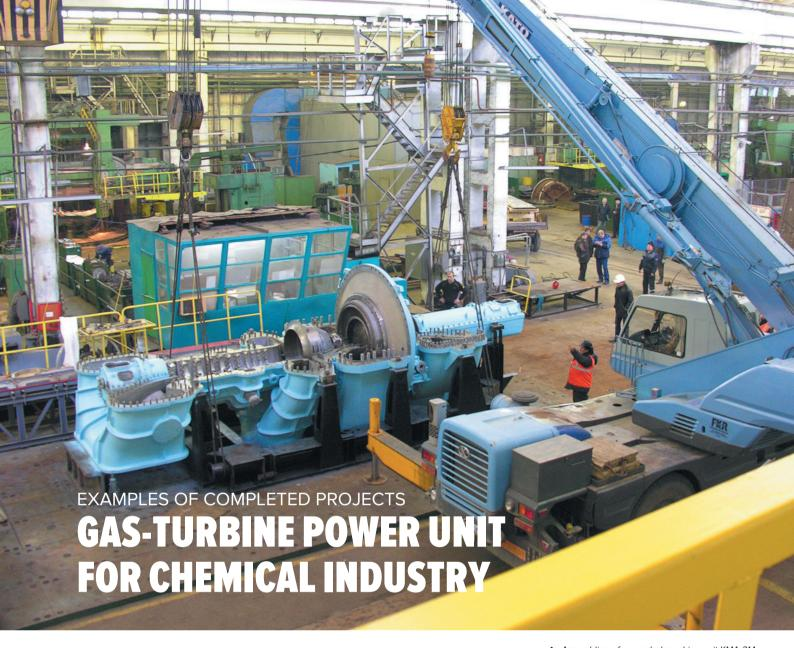
↑ Assembling of upgraded machine unit KMA-2M at the plant 'Dalenergomash'
